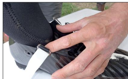
**EN** Check regularly for loose screws. Use a medium-strength threadlocker for the screws on the cuff and on the lever. Check the sole regularly as an excessively worn sole can seriously damage the carbon shell and such damage will not be covered under the warranty.
